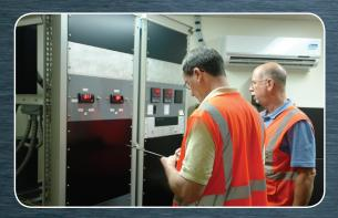
A state-of-the-art computerized data acquisition system collects information from up to 300 sensors used to measure the temperatures, humidity, airflow, and the total energy consumed during the 3-day test period. The results are expressed as the actual U-factor performance of the assembly.
